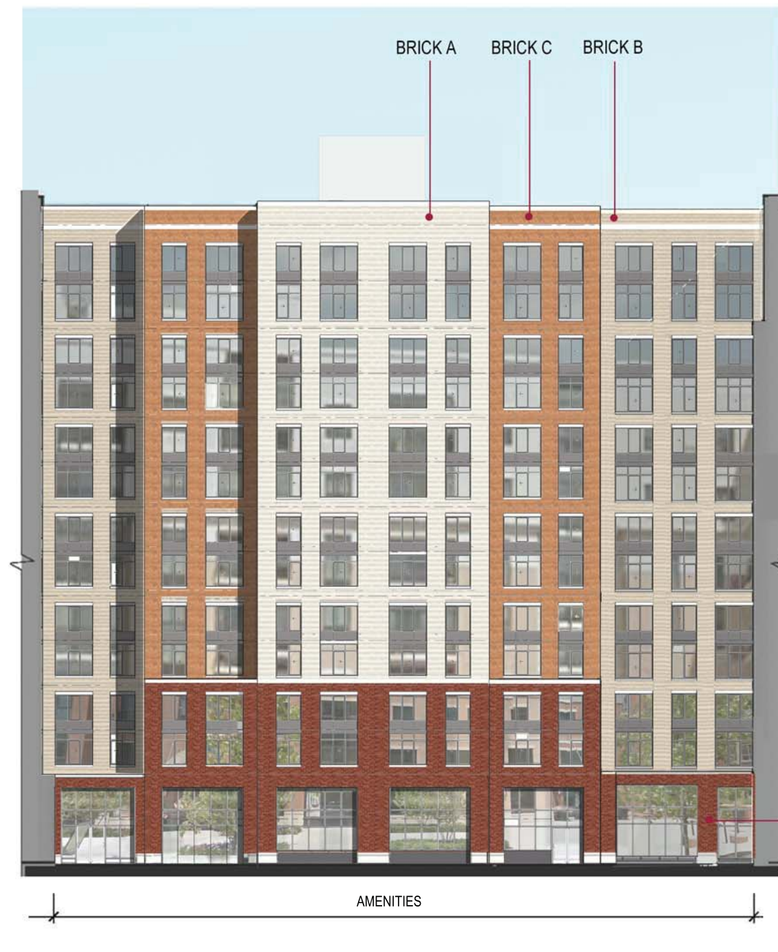
COURTYARD EAST ELEVATION
