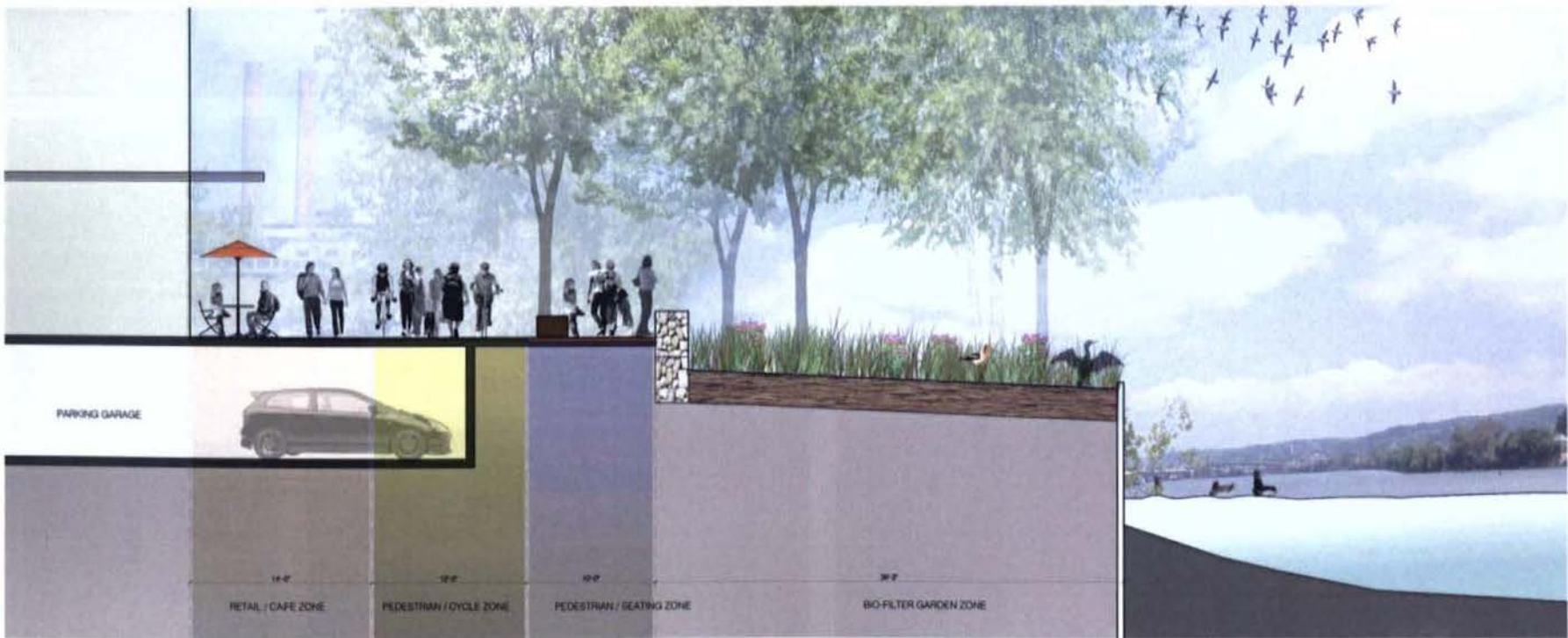
Esplanade Section – at Bio-Filter
