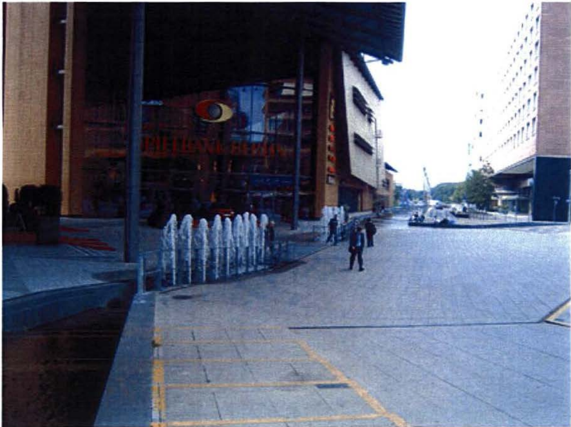
Fountains provide additional water quality improvement through aeration.
