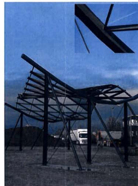
Below & Right: Photographs of the full-scale mock-up from a typical section of the roof, installed at seele Gersthofen in December 2007.
