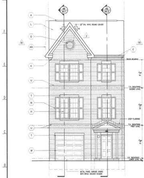
ELEVATION BRICK VENEER W/ BRICK SOLIDER 1/4" = 1'-0" A14
