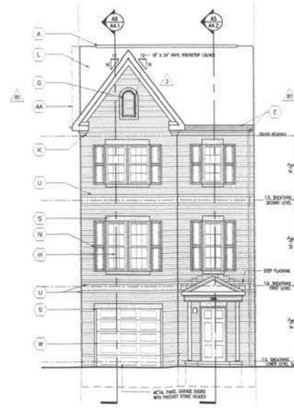
ELEVATION BROOK VENEER W/ STONE HEAD 1/4" x 1'-0"
