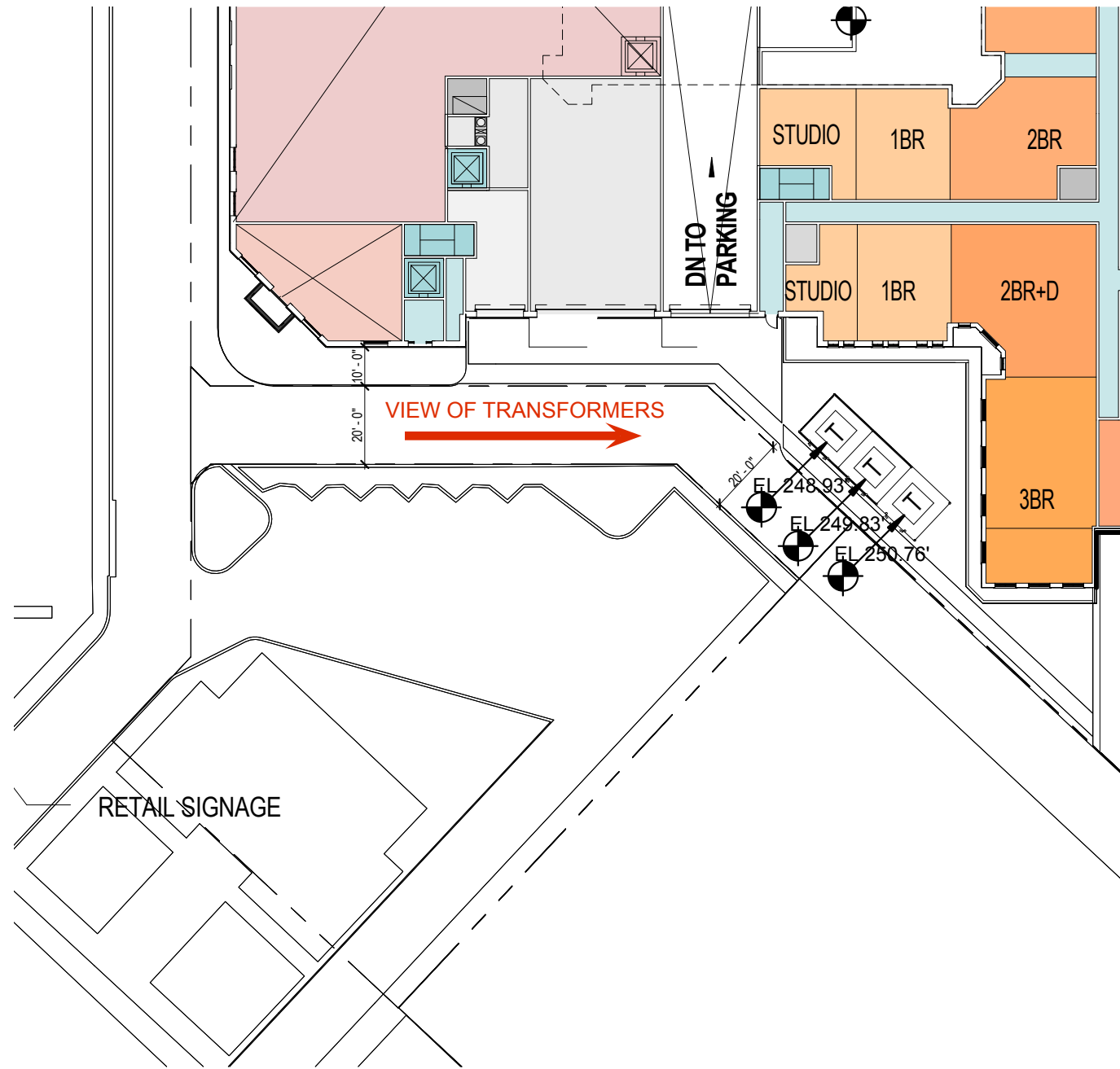
LOWER LEVEL PLAN SHOWING SCREENING FOR TRANSFORMERS
