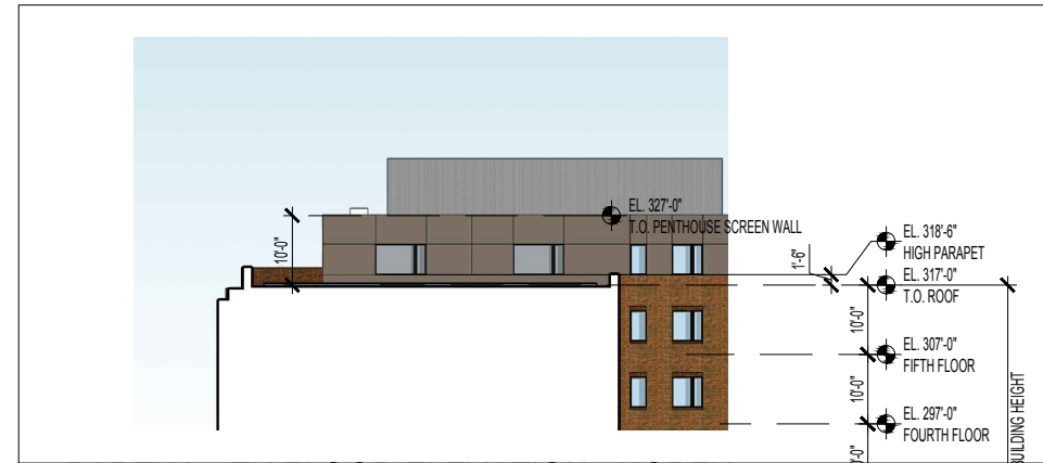
PARTIAL 5TH FLOOR ELEVATION - NORTH
