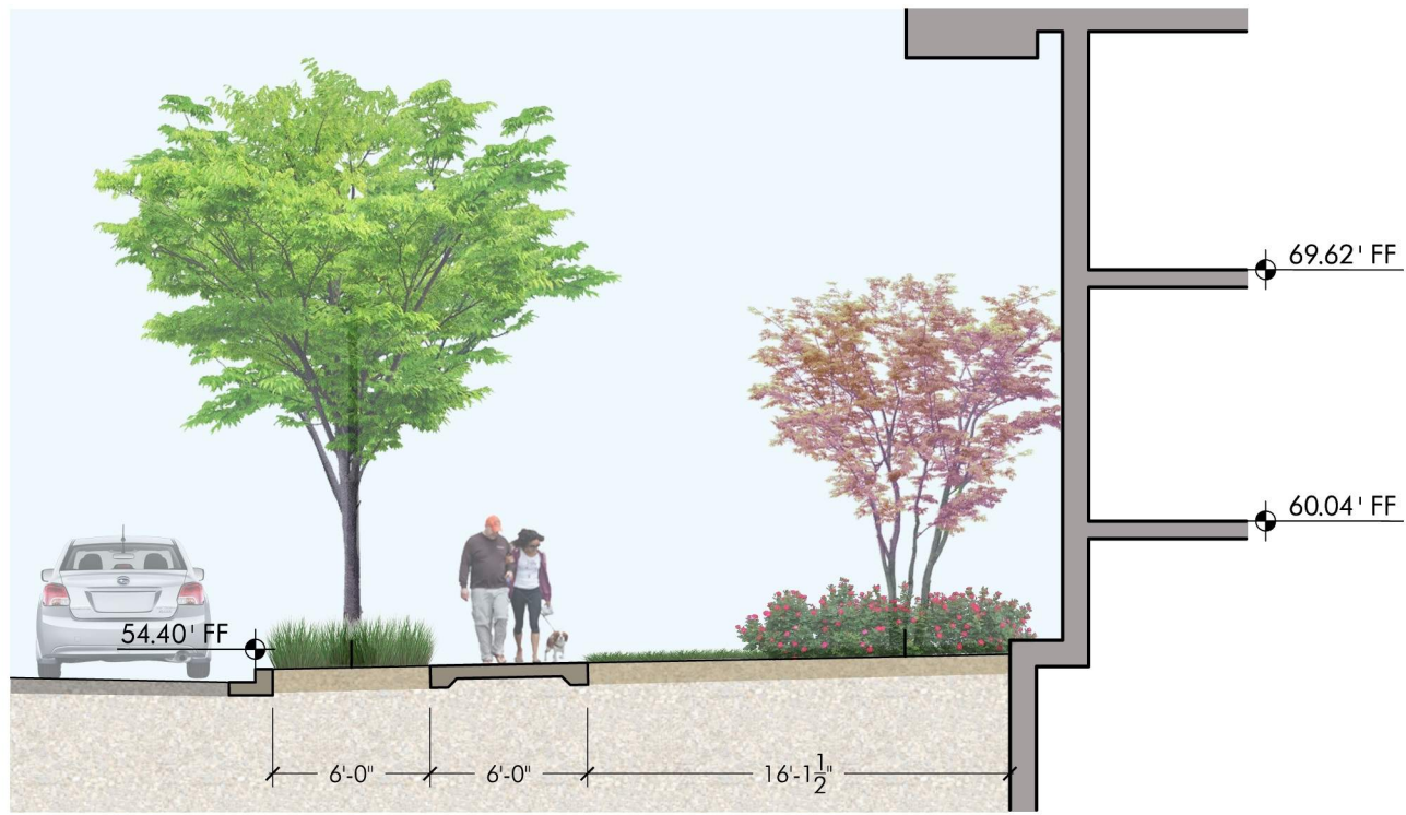
SECTION 1 - 1ST STREET NW SCALE: 1/8"=1'-0"
