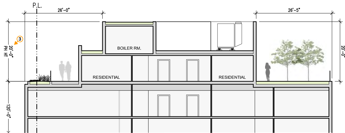
Ⓑ - SOUTH / NORTH ROOFTOP SECTION
