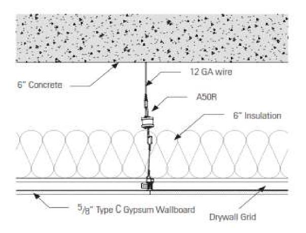
District Dogs sound ceiling detail constructed above dog areas and to be constructed at 907 Barry Place, NW.
