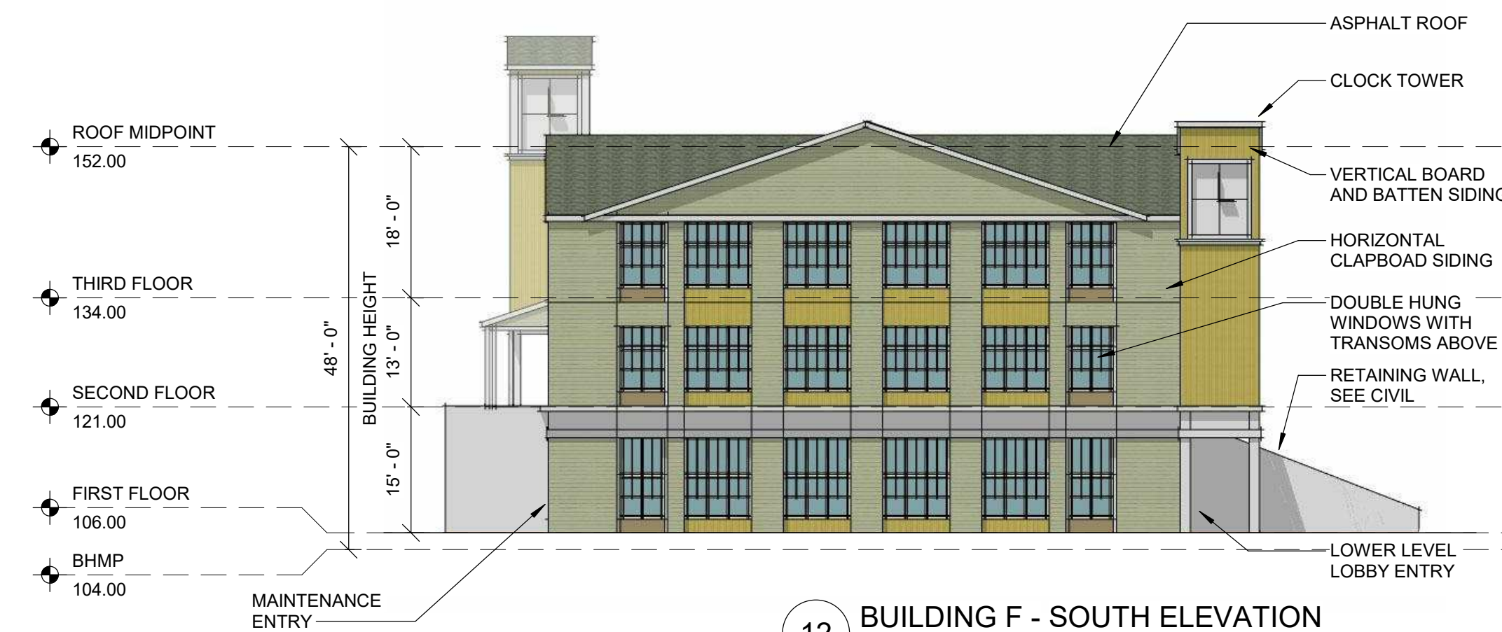
12 BUILDING F - SOUTH ELEVATION
