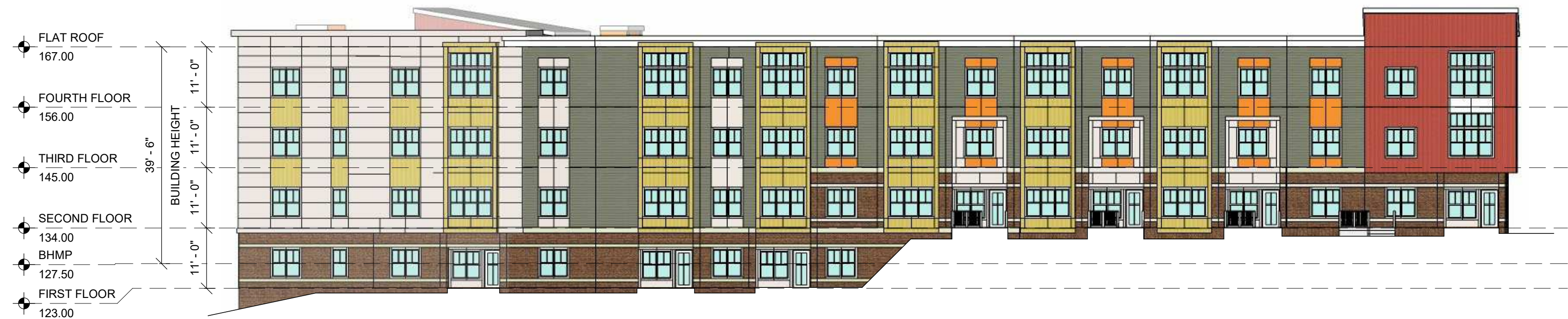
12 BUILDING D - EAST ELEVATION
