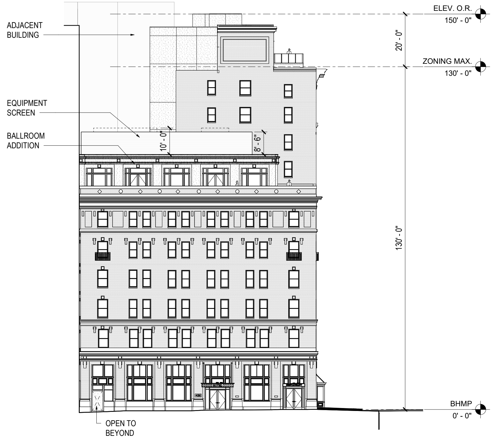
① EXTERIOR ELEVATION - EAST (11TH STREET) 3/64" = 1'-0"
