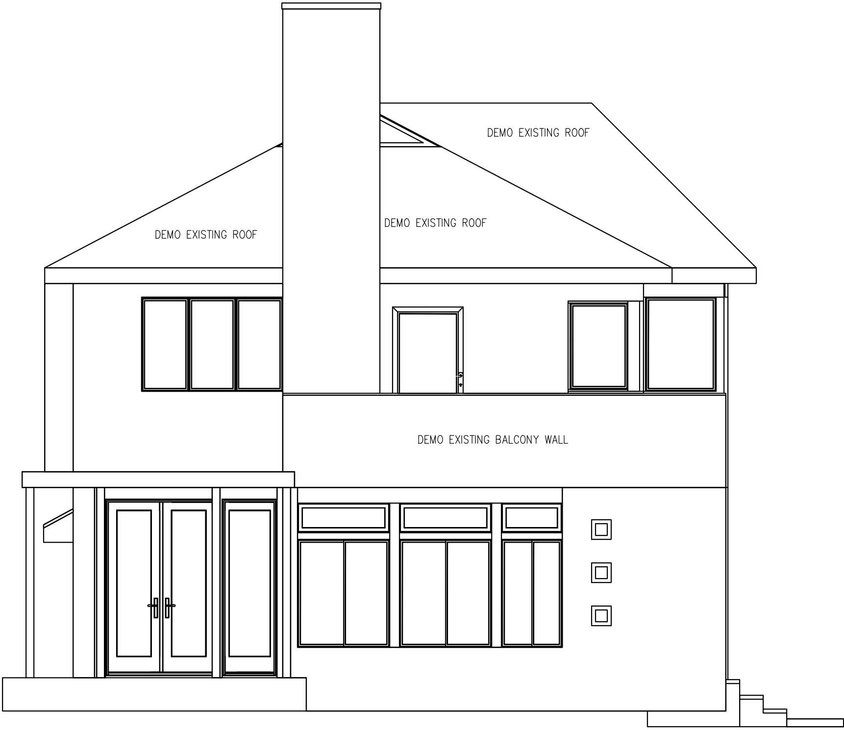
2 ASBUILT EXTERIOR ELEVATION - LEFT SIDE 1/4" = 1'-0"
