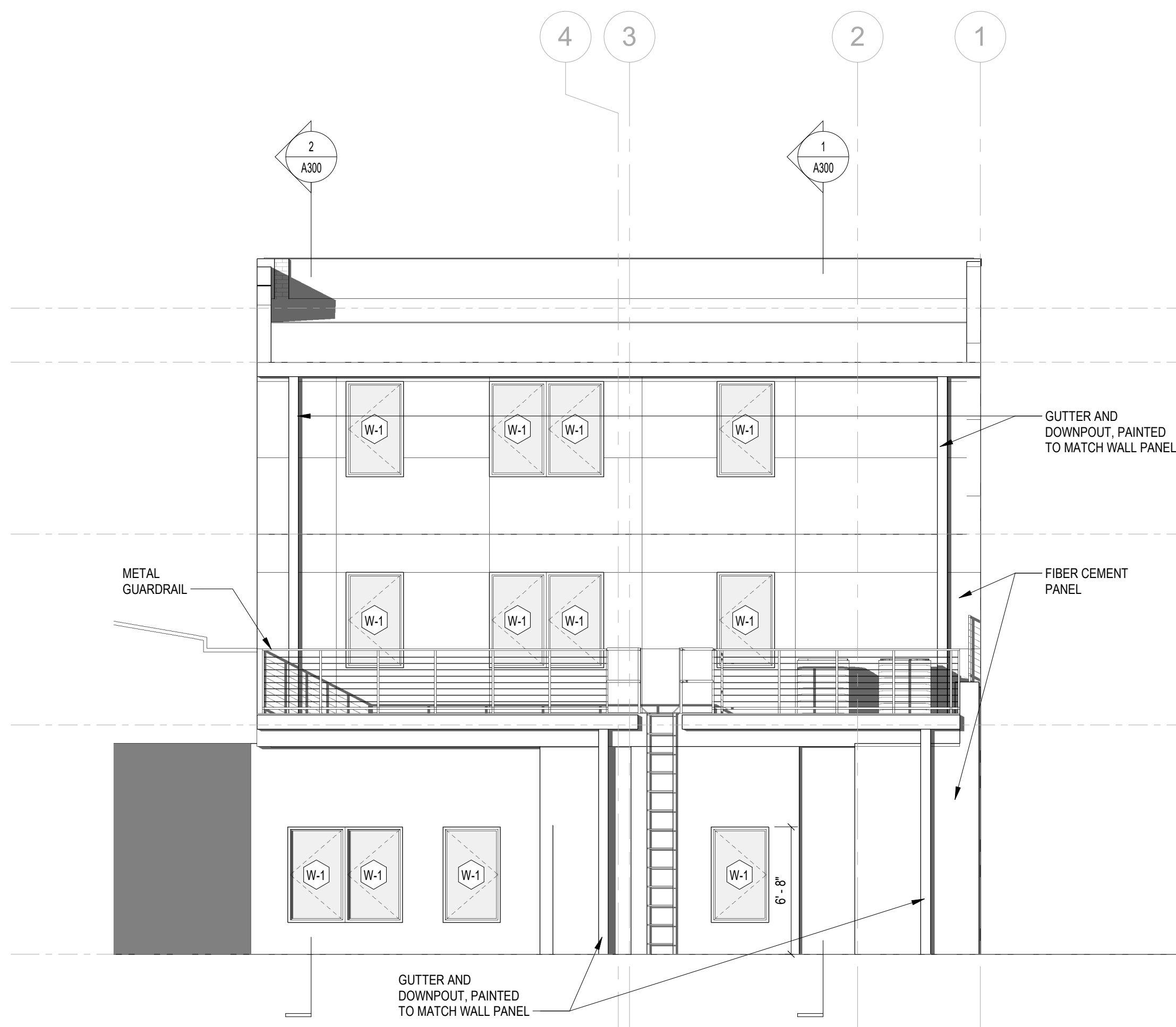
3 REAR ELEVATION (NORTH SIDE) 1 A101 3/16" = 1'-0"
