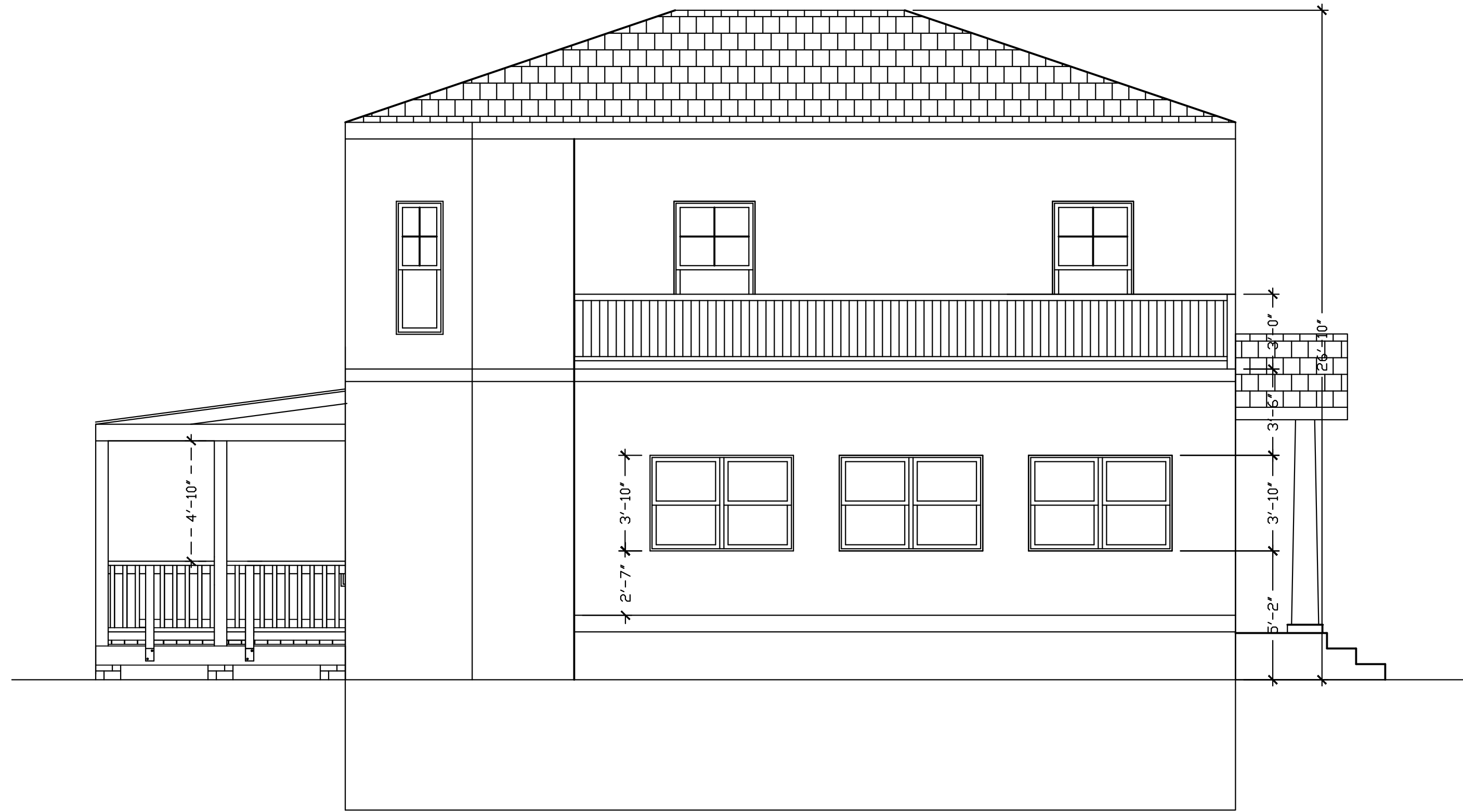
Building Left Side Elevation Scale: 1/4" = 1'-0"
