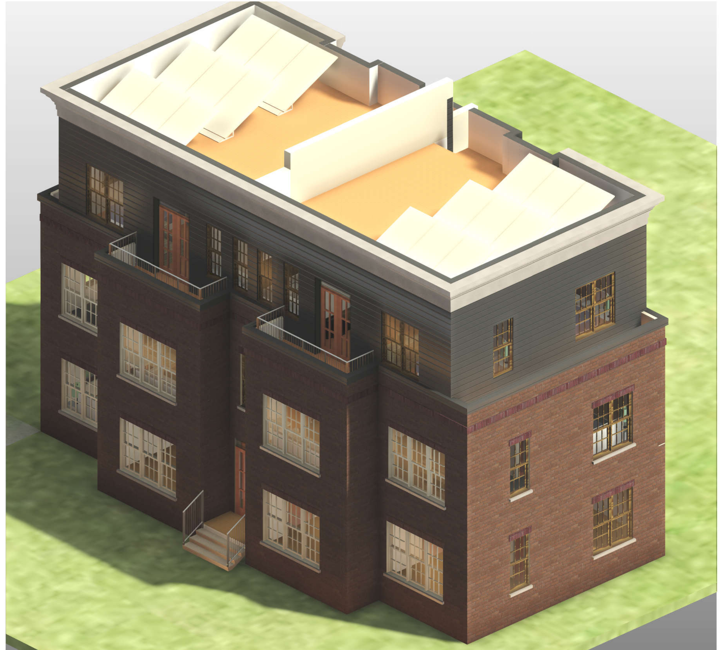
2 SOUTH EAST ISOMETRIC VIEW OF PROPOSED 3RD FLOOR ADDITION WITH OPEN STAIR TO ROOF DECK TERRACE
