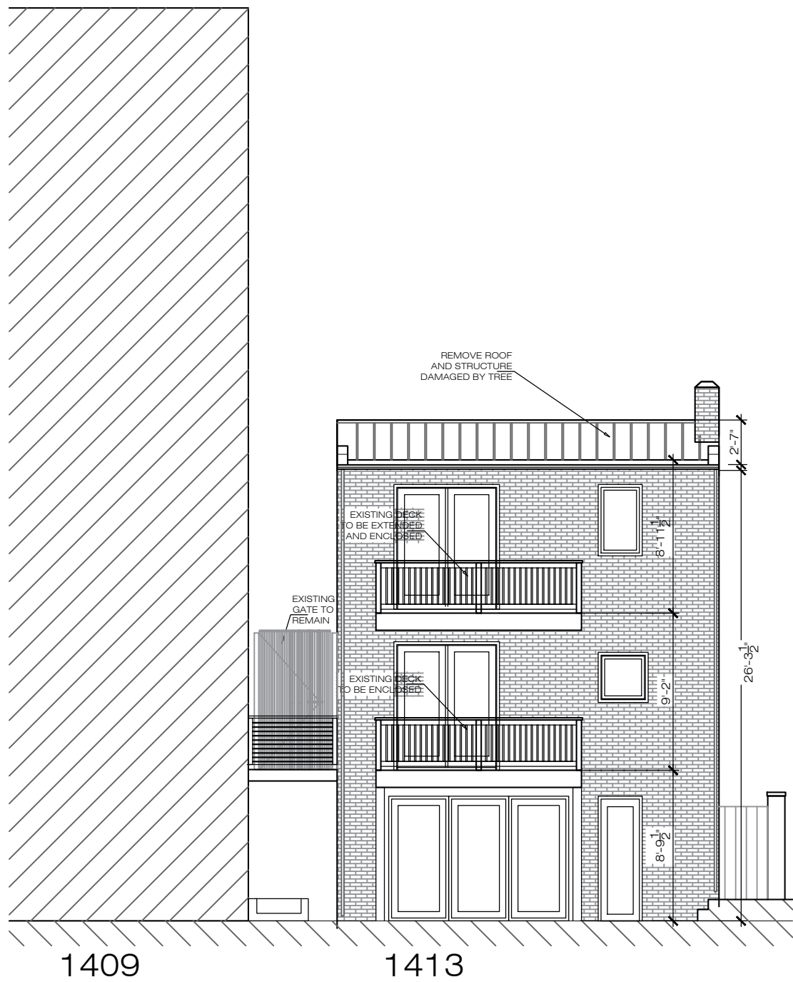
1 EXISTING BACK ELEVATION 1/8" = 1'-0"
