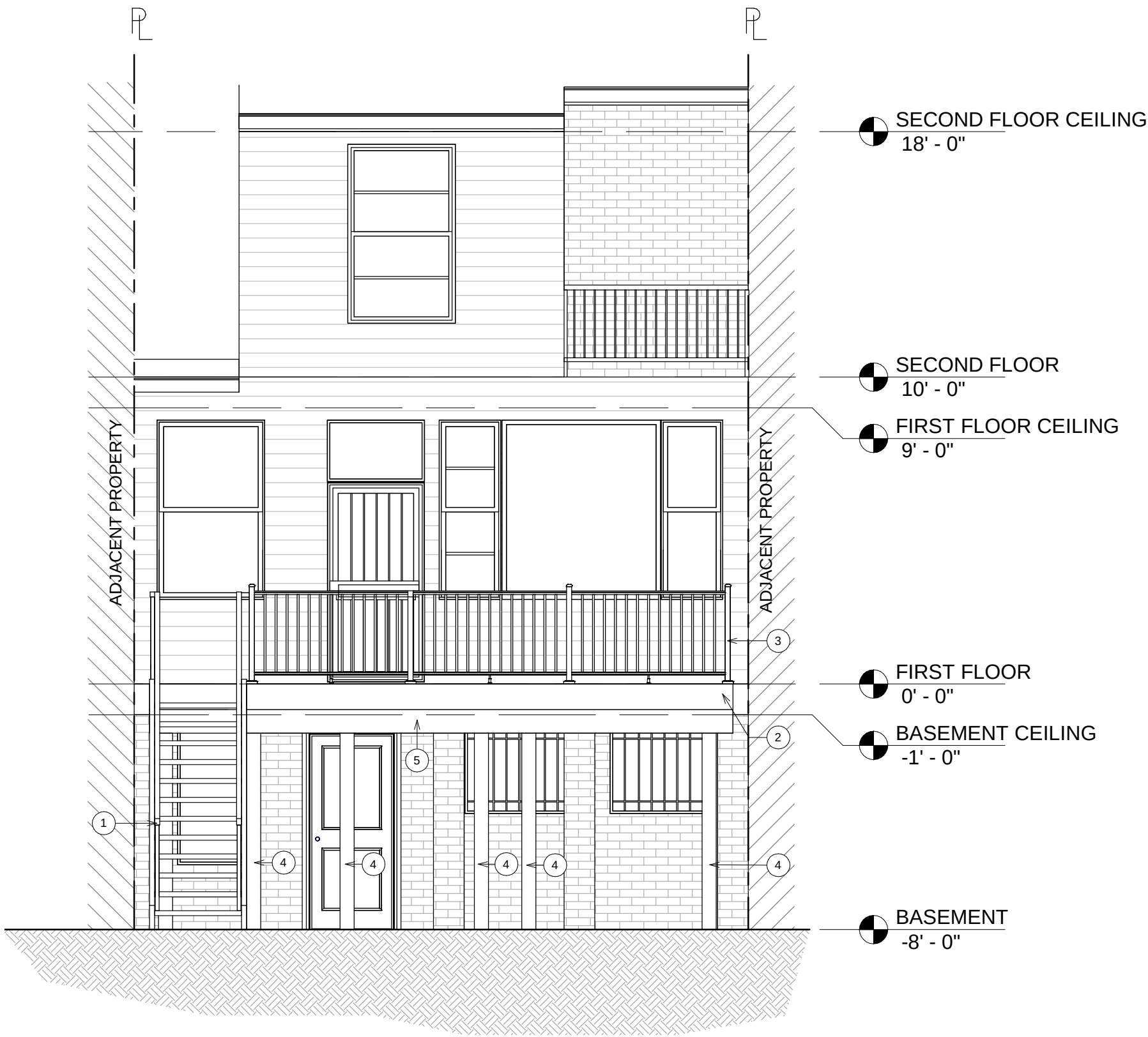
1. PROP. REAR ELEVATION 1/4" = 1'-0"
