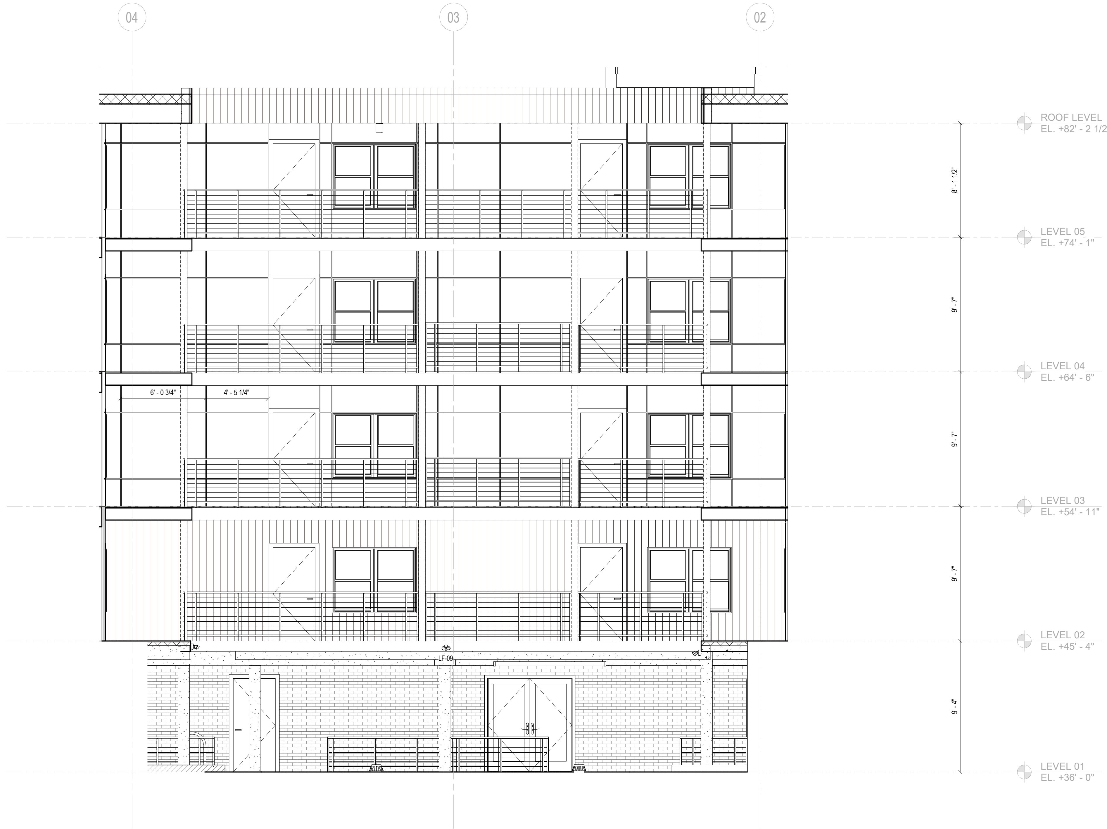
2 ELEVATION - EXTERIOR VIEW F - BZA 1/4" = 1'-0"
