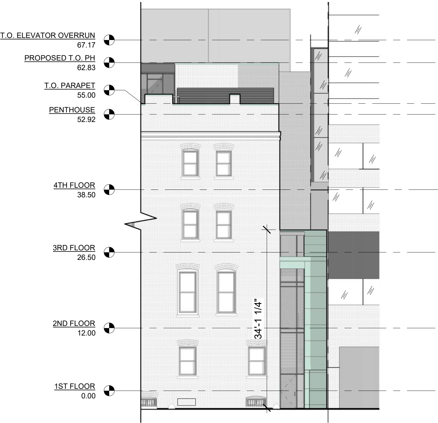
ALLEY ELEVATION AT REAR STAIR ADDITION (NORTH) 3/32" = 1'-0"
