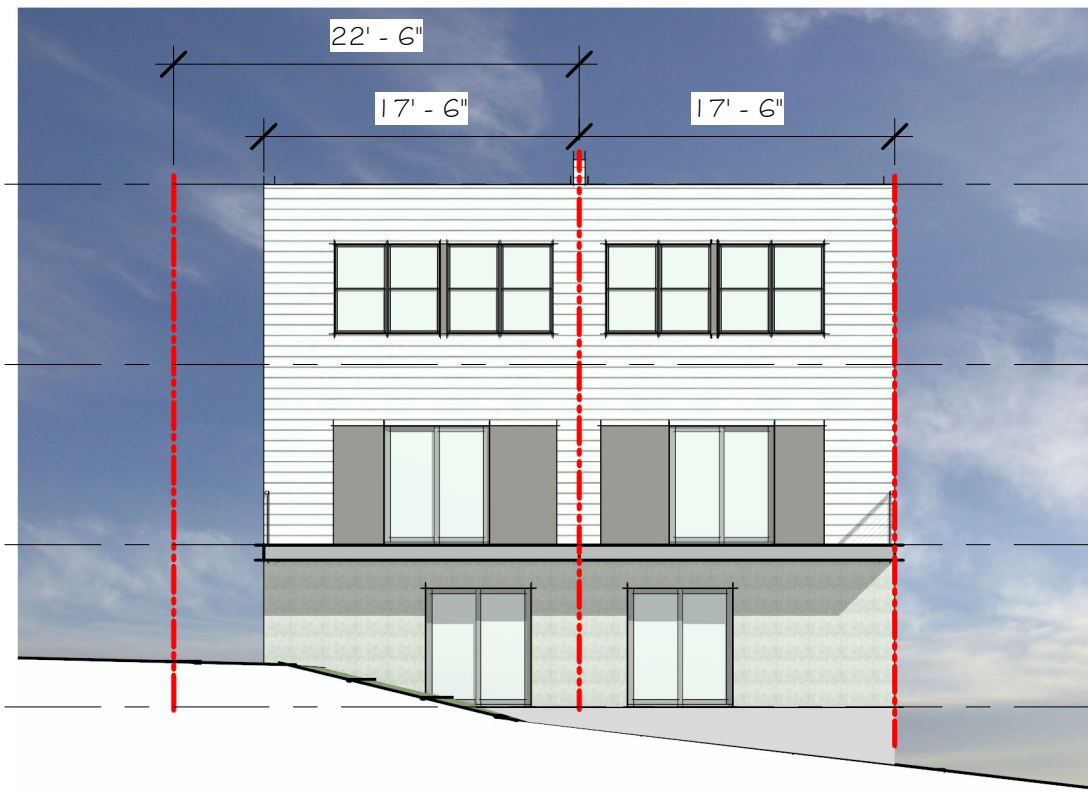
02 SOUTH - REAR ELEVATION SCALE 3/32" = 1'-0"
