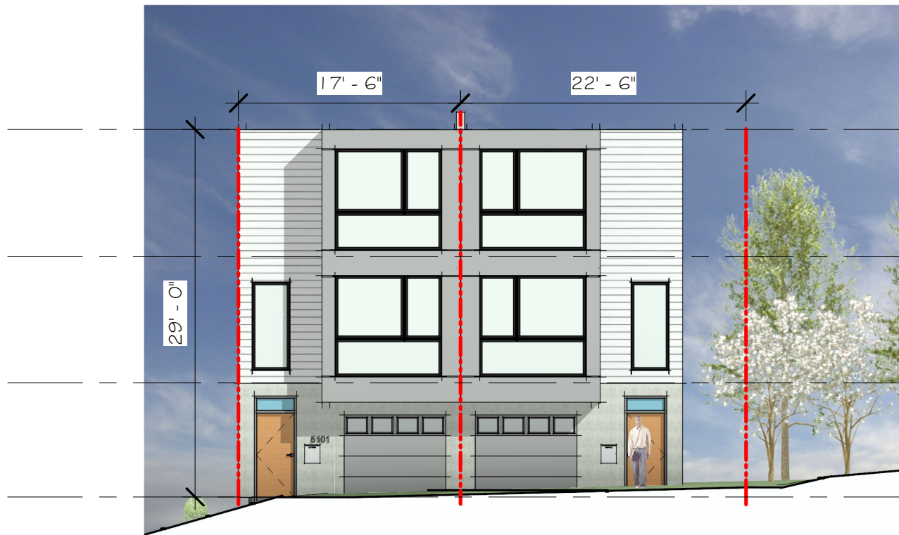
01 SOUTH - FRONT ELEVATION SCALE 3/32" = 1'-0"
