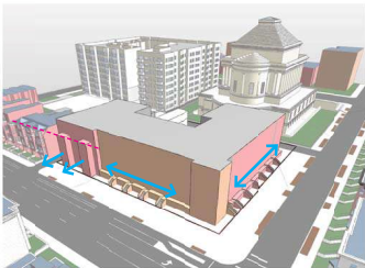
6 INTRODUCE BUILDING BASE AND AND FRAME LOBBY WITH BAYS MATCHING ADJACENT PROPERTIES
