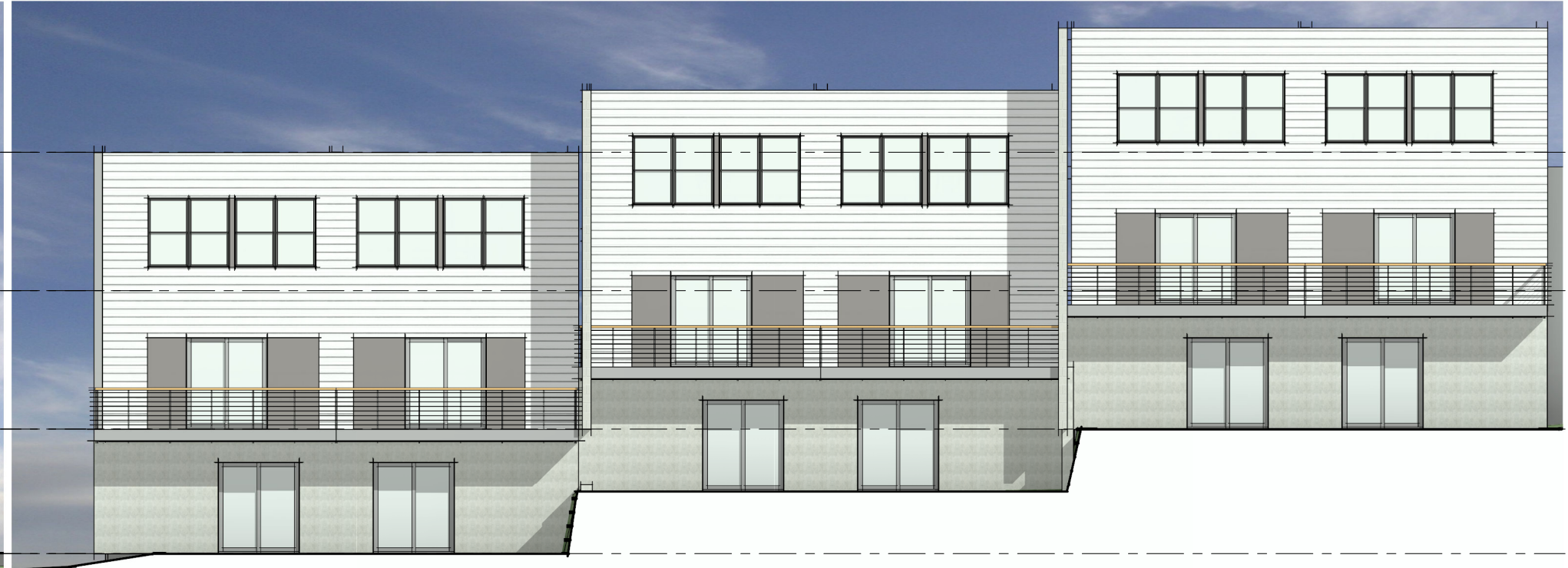
03 North -Back Elevation SCALE 3/32" = 1'-0"
