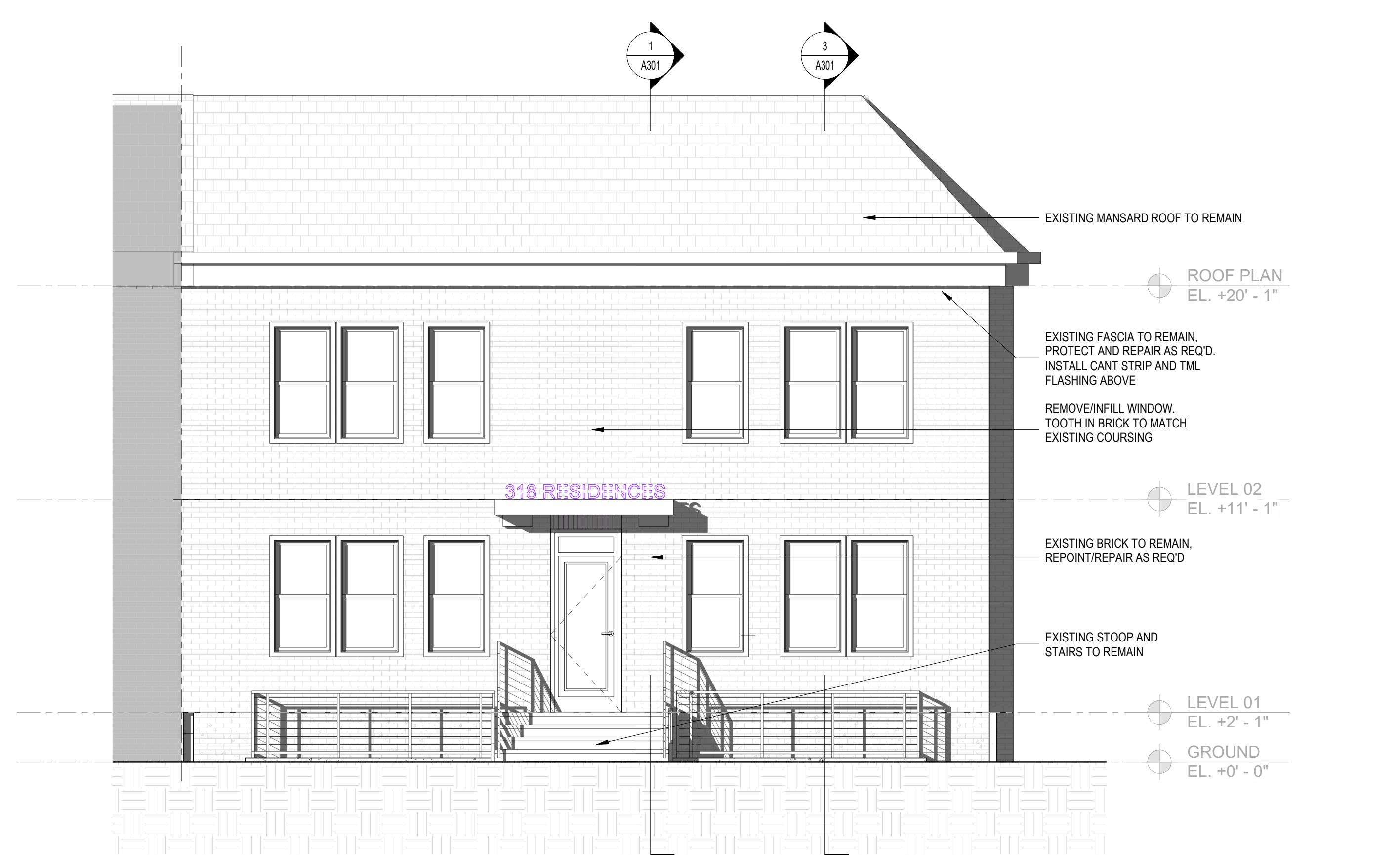
1 FRONT ELEVATION - NEW CONSTRUCTION 1/4" = 1'-0"
