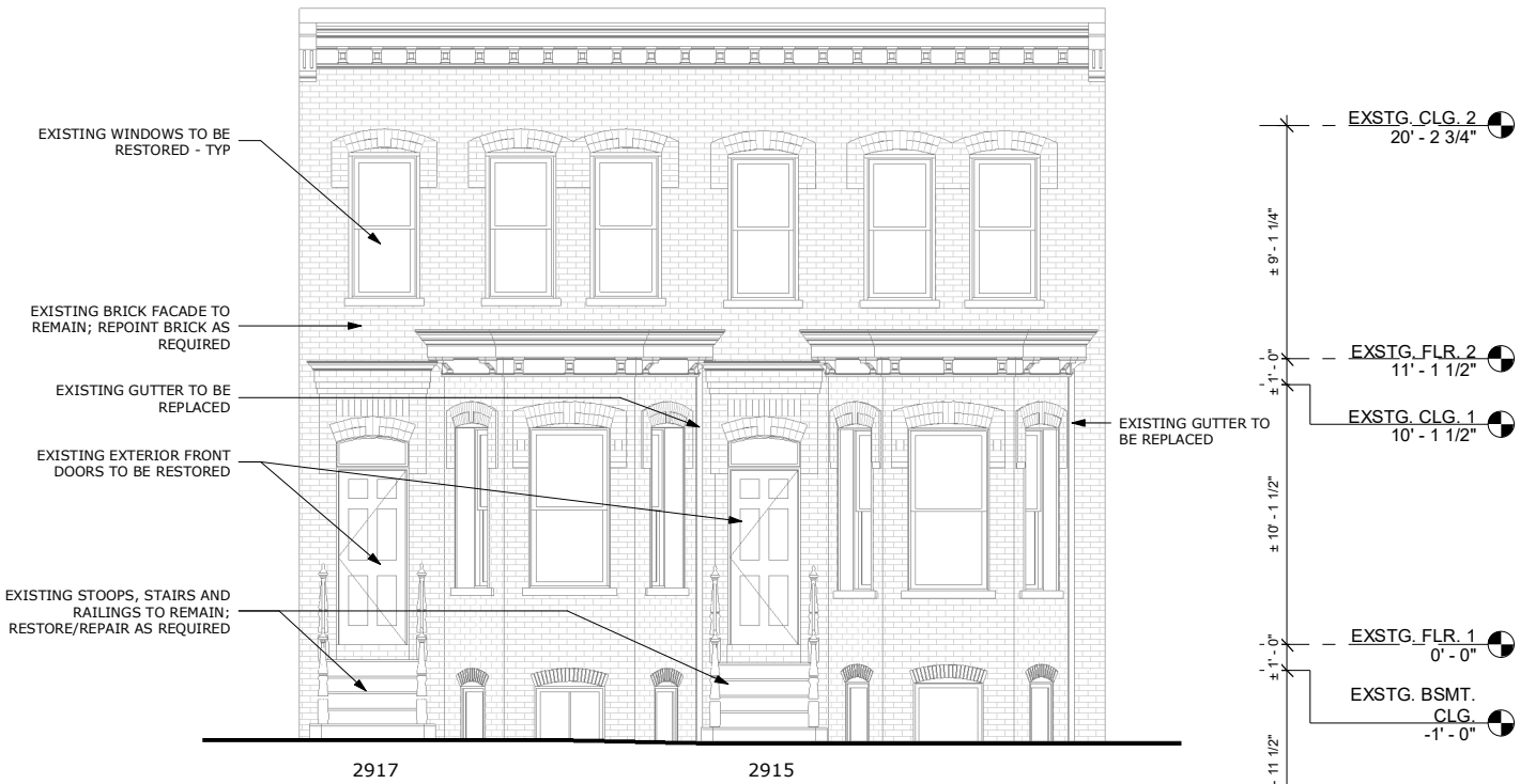
① Proposed Front Elevation 1/8" = 1'-0"
