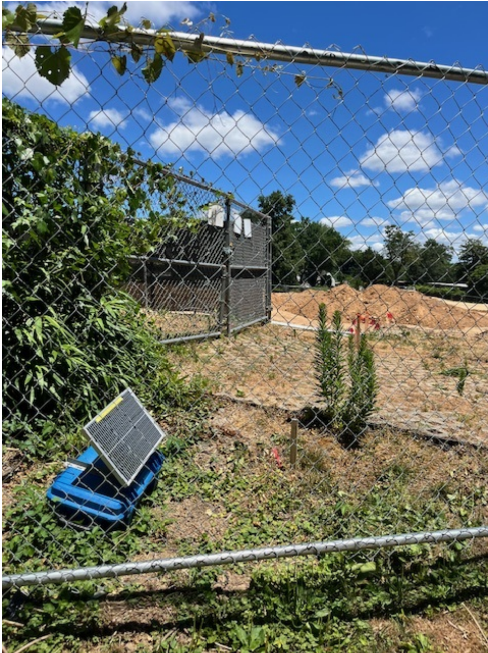
Figure 7: Vibration Monitoring – UM18273
