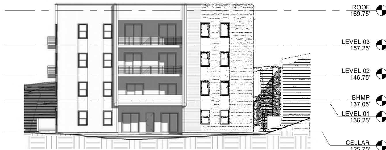
④ EXTERIOR ELEVATION - WEST 1" = 20'-0"
