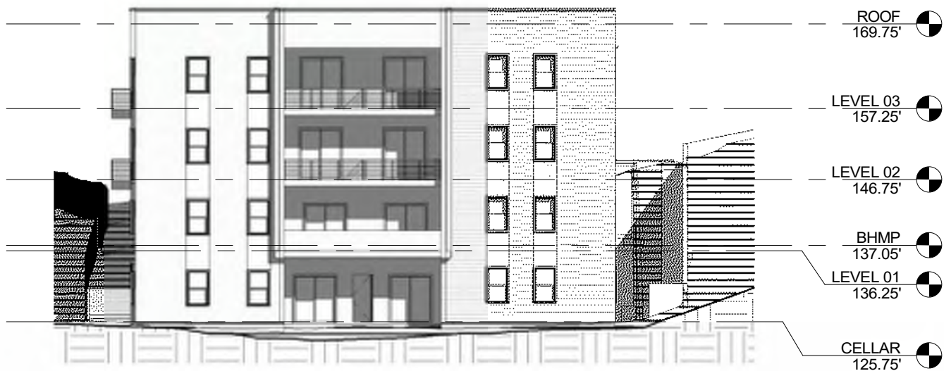
4 EXTERIOR ELEVATION - WEST 1" = 20'-0"
