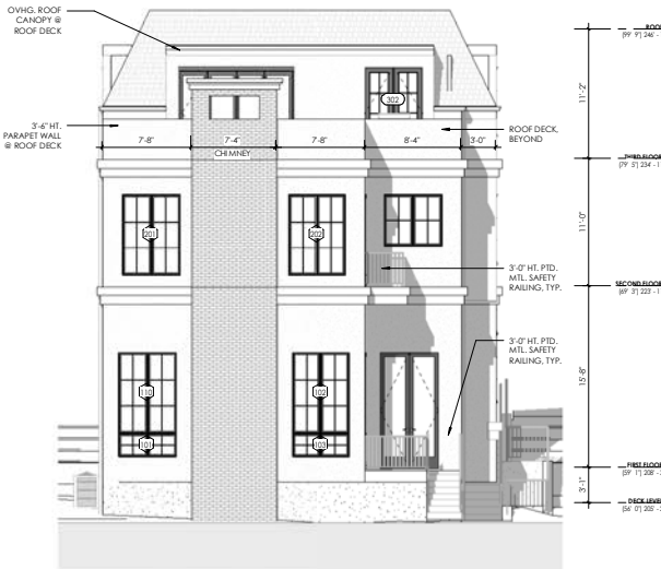
③ REAR ELEVATION (SOUTH) 3/16" = 1'-0"
