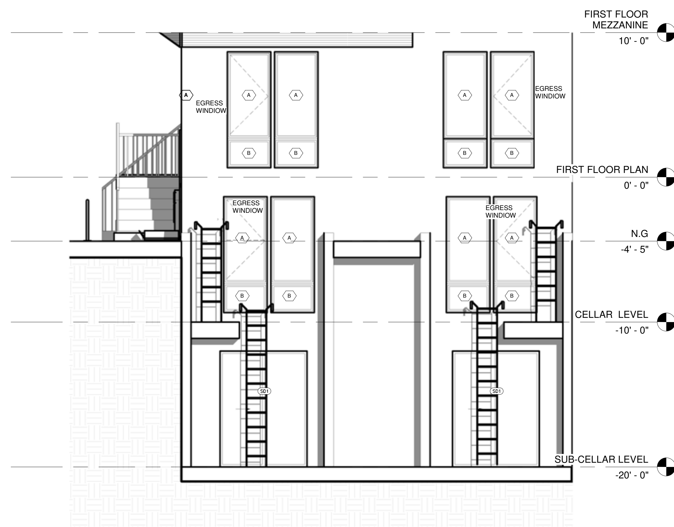
3 FRONT ELEVATION @ AREAWAY 1/4" = 1'-0"
