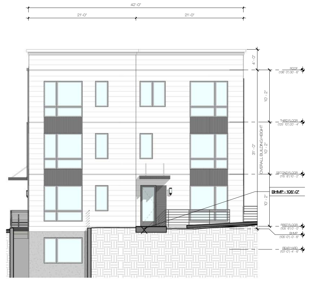
① WEST (LEFT) STREET ELEVATION 3/16" = 1'-0"
