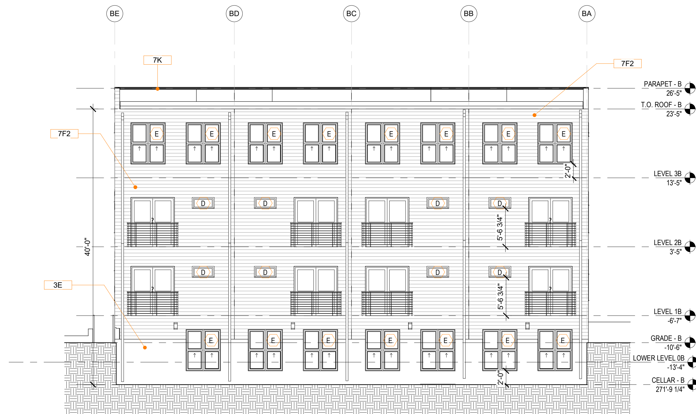
BUILDING B - NORTH ELEVATION
