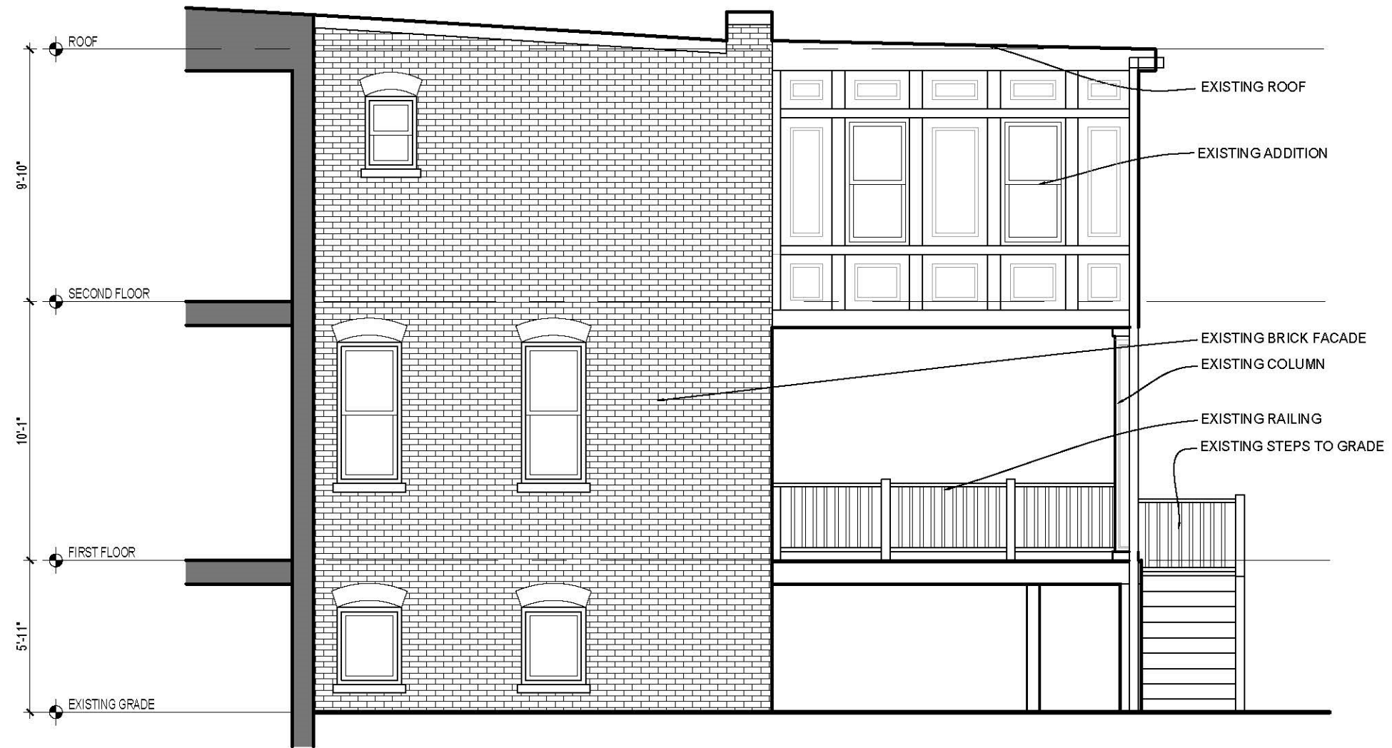
1 EXISTING NORTH ELEVATION D-4 SCALE: 3/16"=1'-0"
