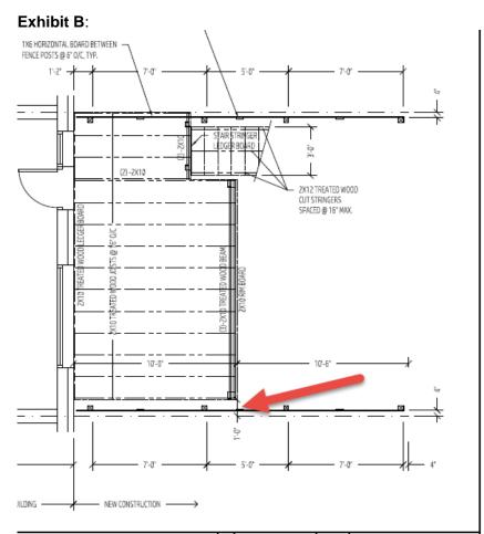
We modified the width of the deck from the neighbors property line from 3.5 inches to a one foot, ensuring there is ample distance to allow the line of sight to not be obstructed.
