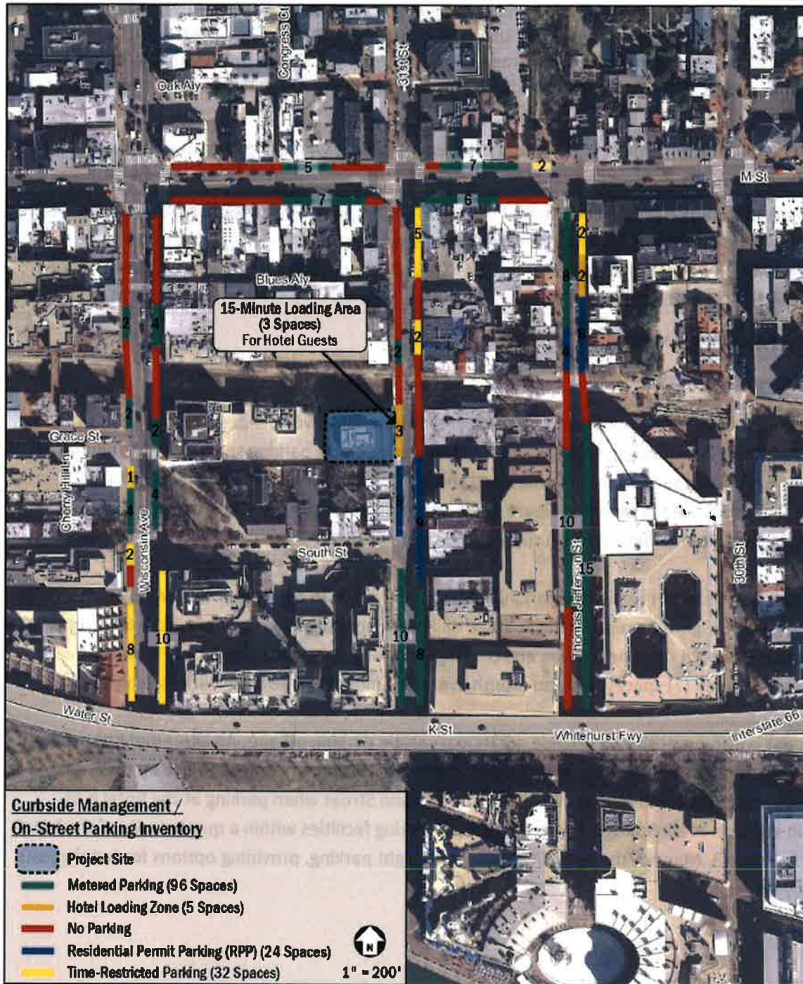
Figure 1. Inventory of Curbside Management and On-Street Parking (Source: Gorove/Slade, CTR, Figure 8, 6/10/2019)
