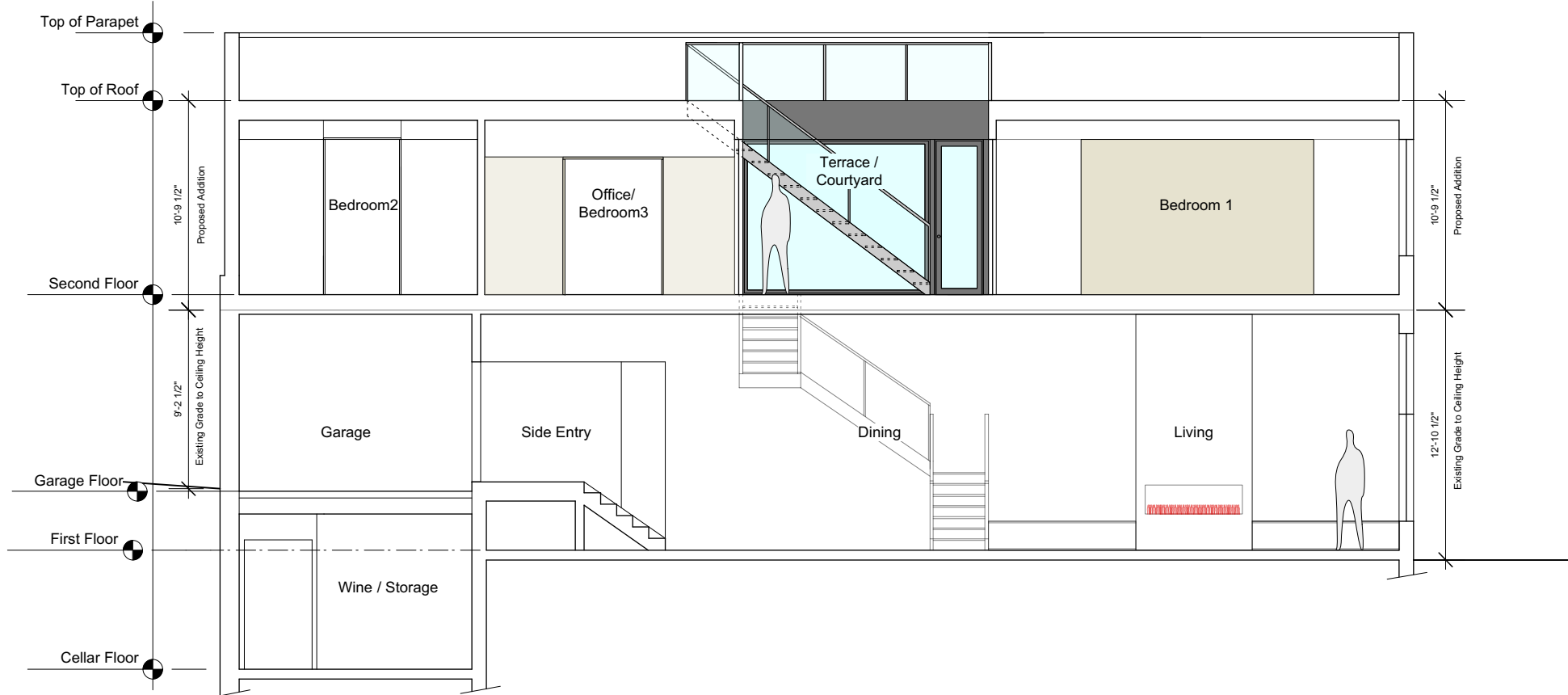
Proposed Building Section 2 scale: 1/8" = 1'-0"
