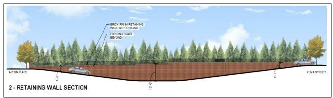
On the eastern portion of the site, a driveway ramp with an entrance from Alton Place and egress on Yuma Street is proposed to provide access to the below grade parking and loading. To access the below grade garage, a ramp with an acceptable slope must be provided. The inward facing retaining wall along the sides of the ramp would therefore, over part of its length, exceed the maximum permitted height.
