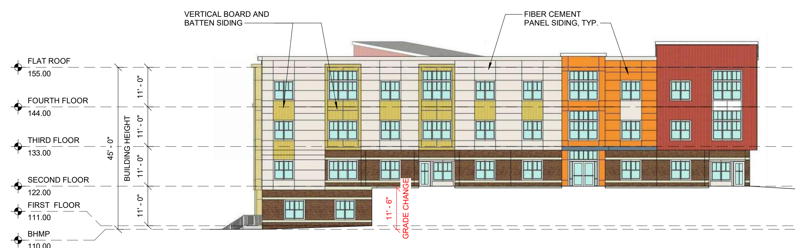
10 BUILDING E - NORTH ELEVATION
