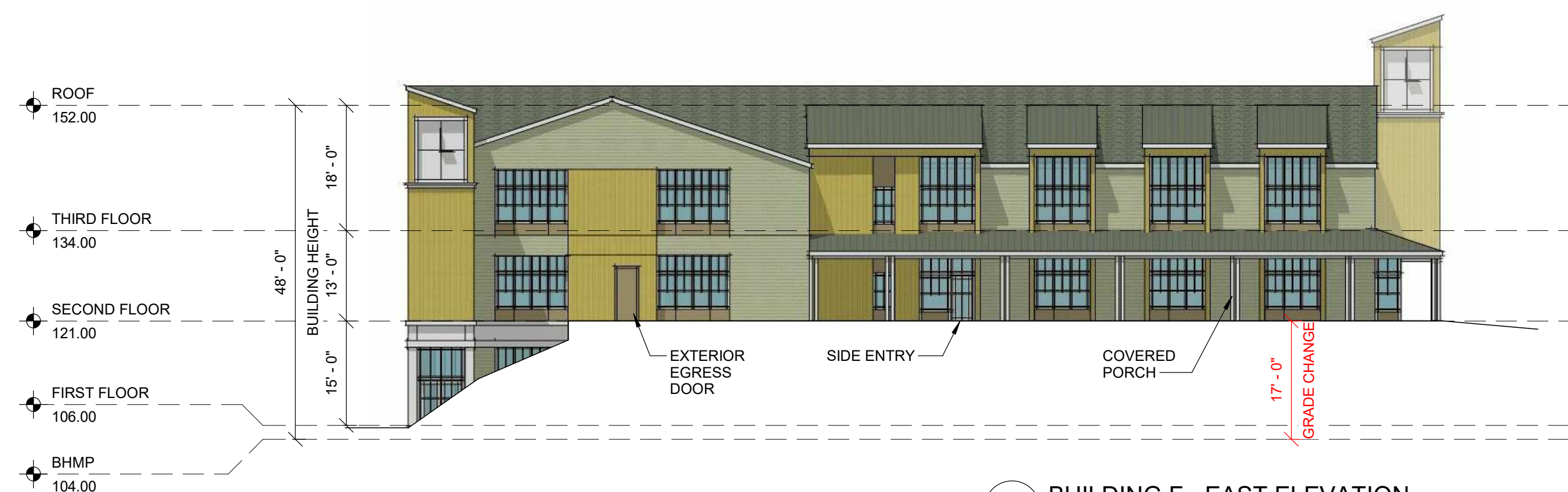
11 BUILDING F - EAST ELEVATION
