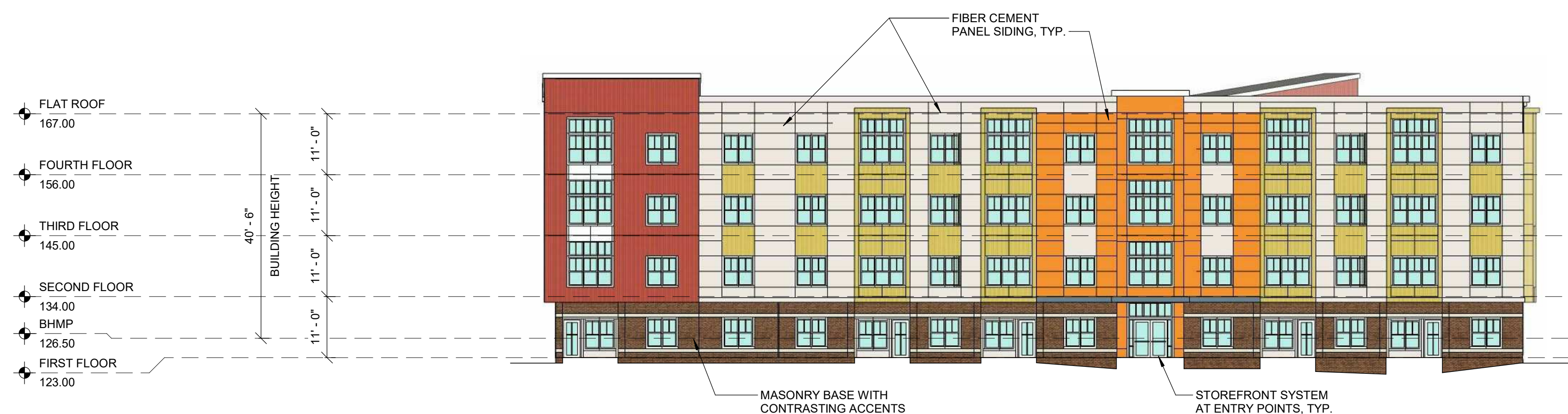
12 BUILDING D - SOUTH ELEVATION
