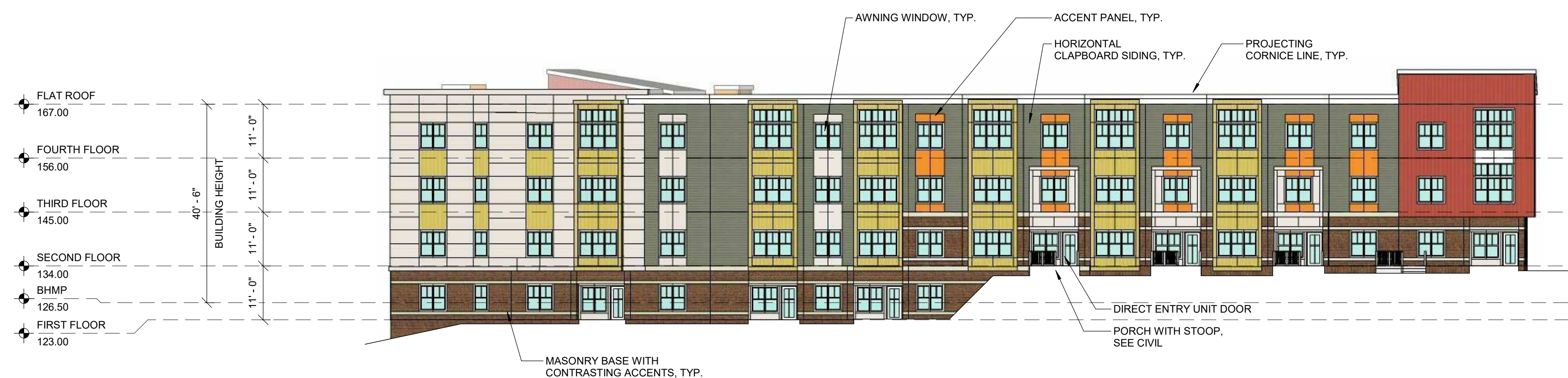
11 BUILDING D - EAST ELEVATION
