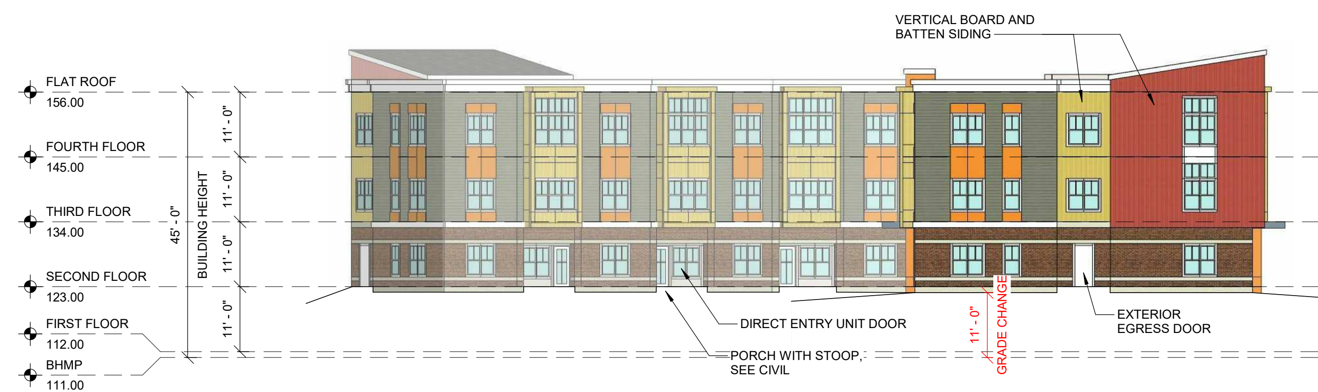
11 BUILDING H - EAST ELEVATION
