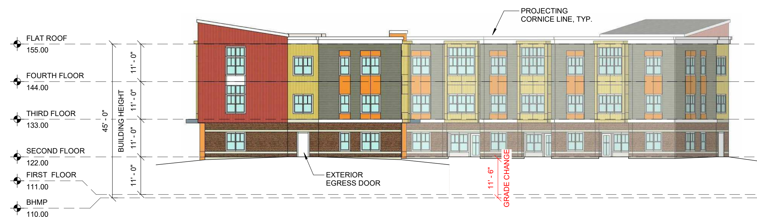
13 BUILDING E - WEST ELEVATION
