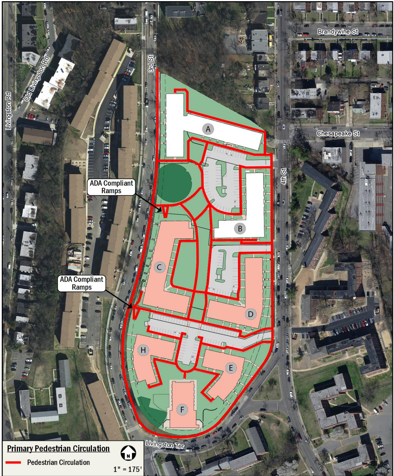
Figure 4: Pedestrian Site Circulation
