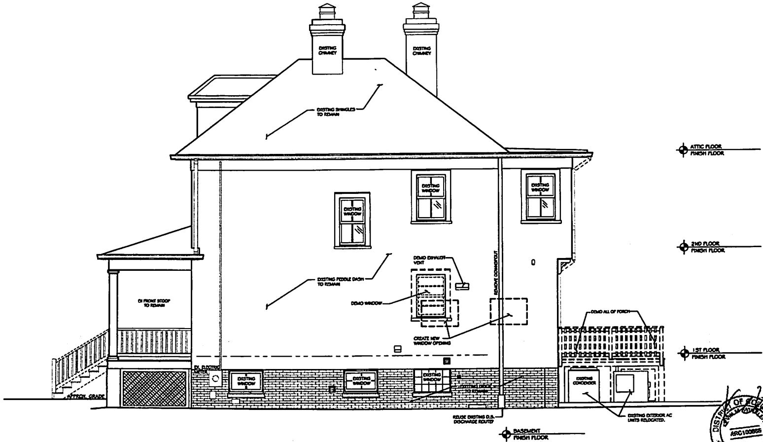
1 DEMOLITION- EXTERIOR ELEVATION SCALE: 1/4"=1'-0"
