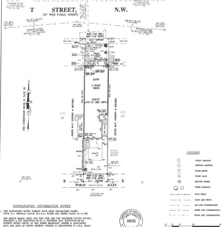
SMH S&A #503 TOP ELEVATION = 89.72 SMH S&A #504 TOP ELEVATION = 88.47
