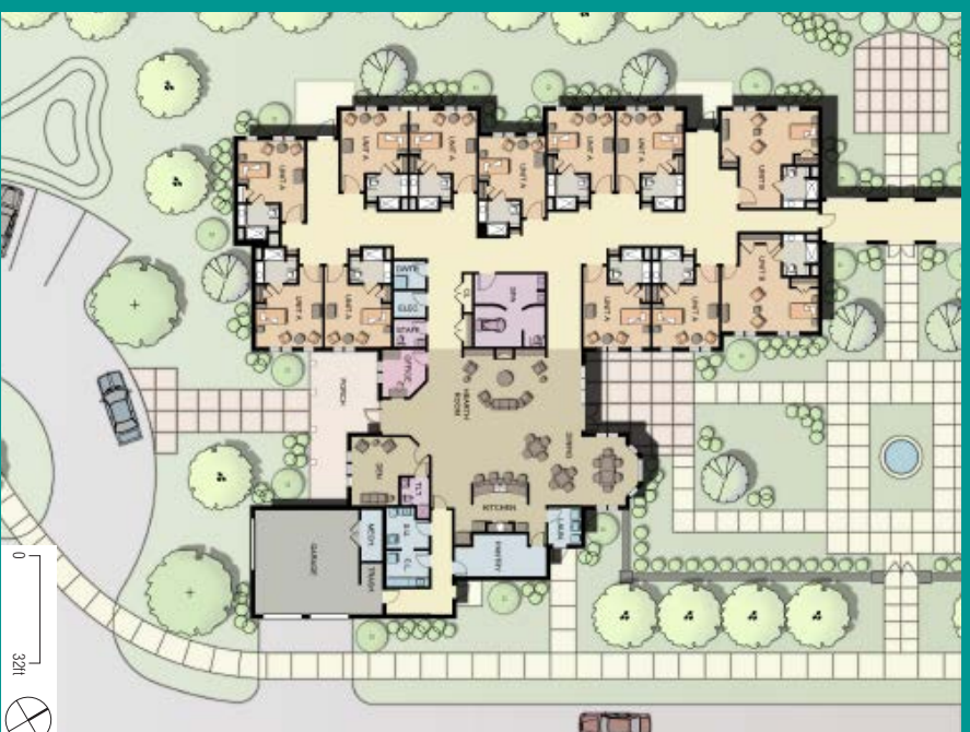
Several DFAR12 projects, like The Deupree House and Nursing Cottages, are reworking the layout of the Household for a better hierarchy of public-to-private spaces. Bedrooms no longer open into common areas, like living or dining rooms.
