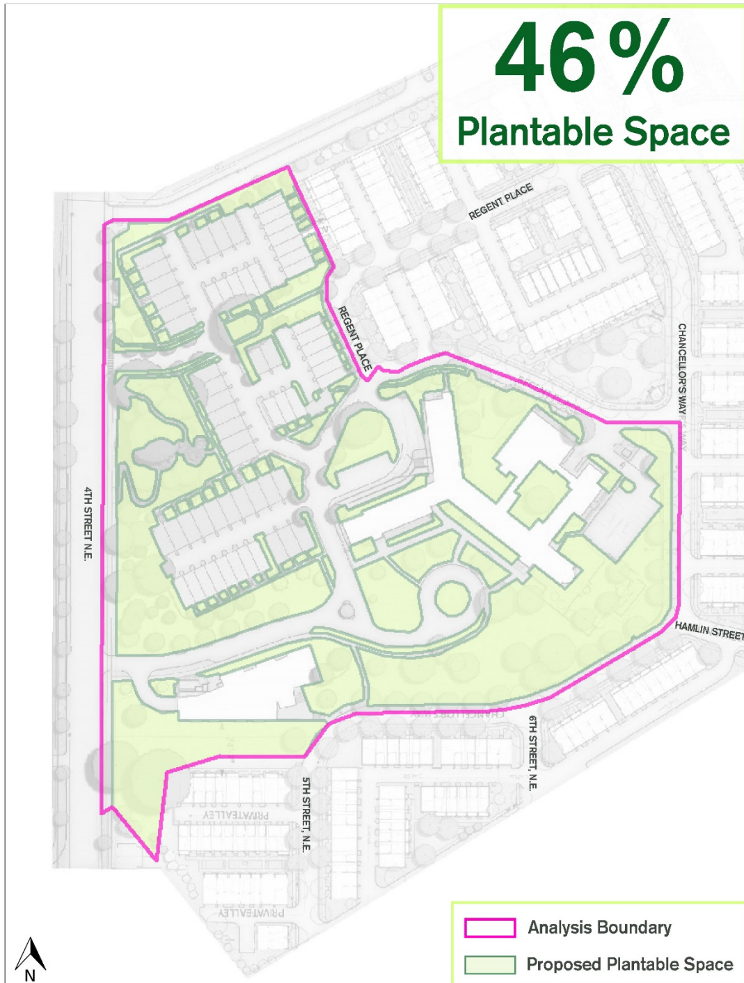
Figure 5. After townhomes are constructed, 46% of the entire site will remain plantable space. This provides the necessary space to plant replacement trees and achieve a 30% tree canopy goal.
