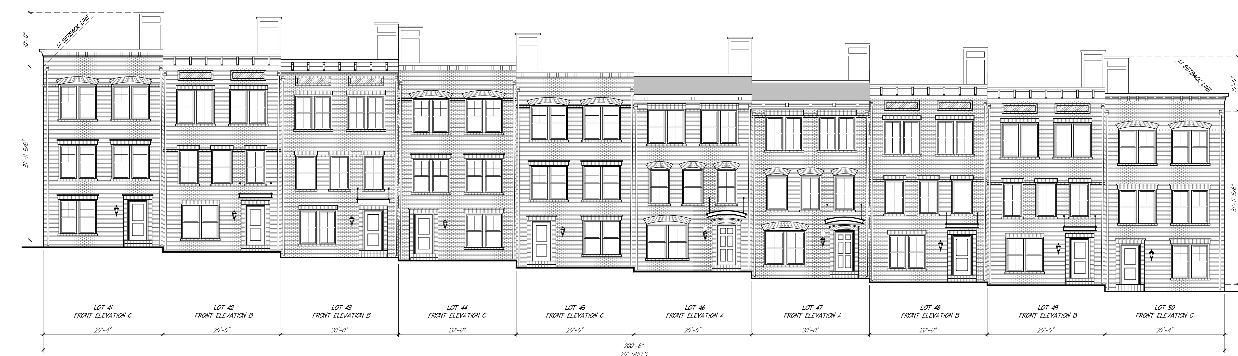
BUILDING ELEVATIONS - LOTS # 41-50 SCALE: 1/8" = 1'-0"
