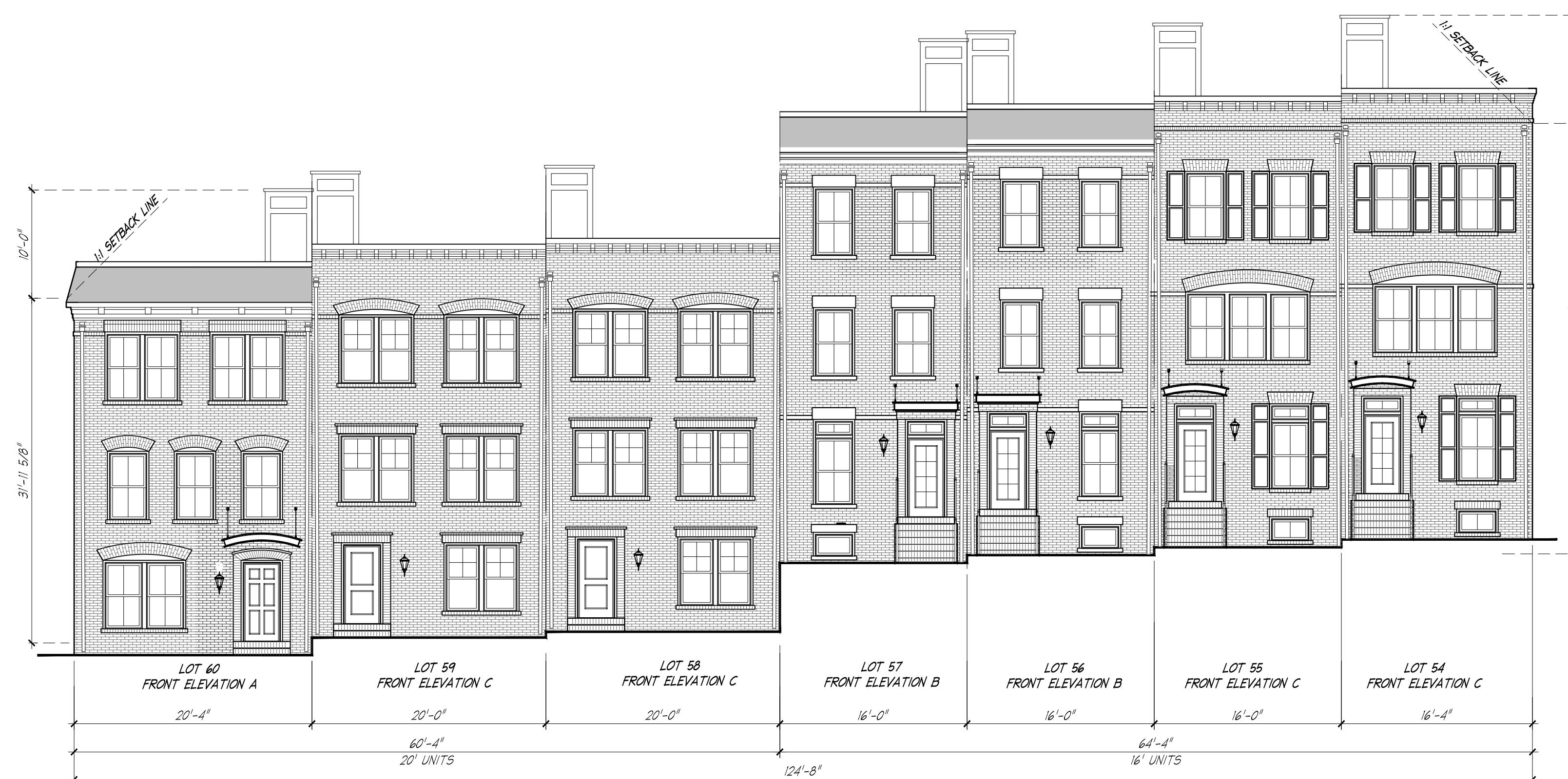
01 BUILDING ELEVATIONS - LOTS # 60-54 A17 SCALE: 1/8" = 1'-0"
