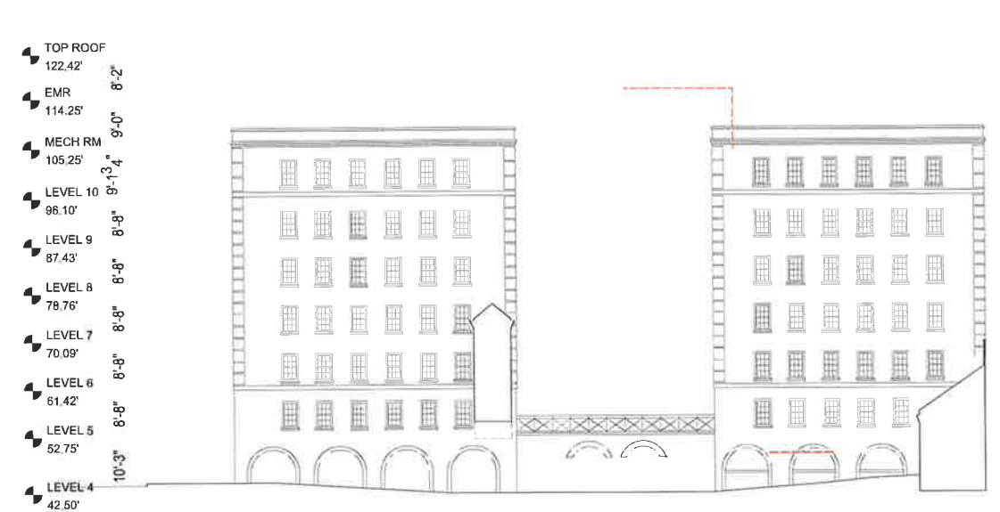
3. NORTH COURTYARD ELEVATION
