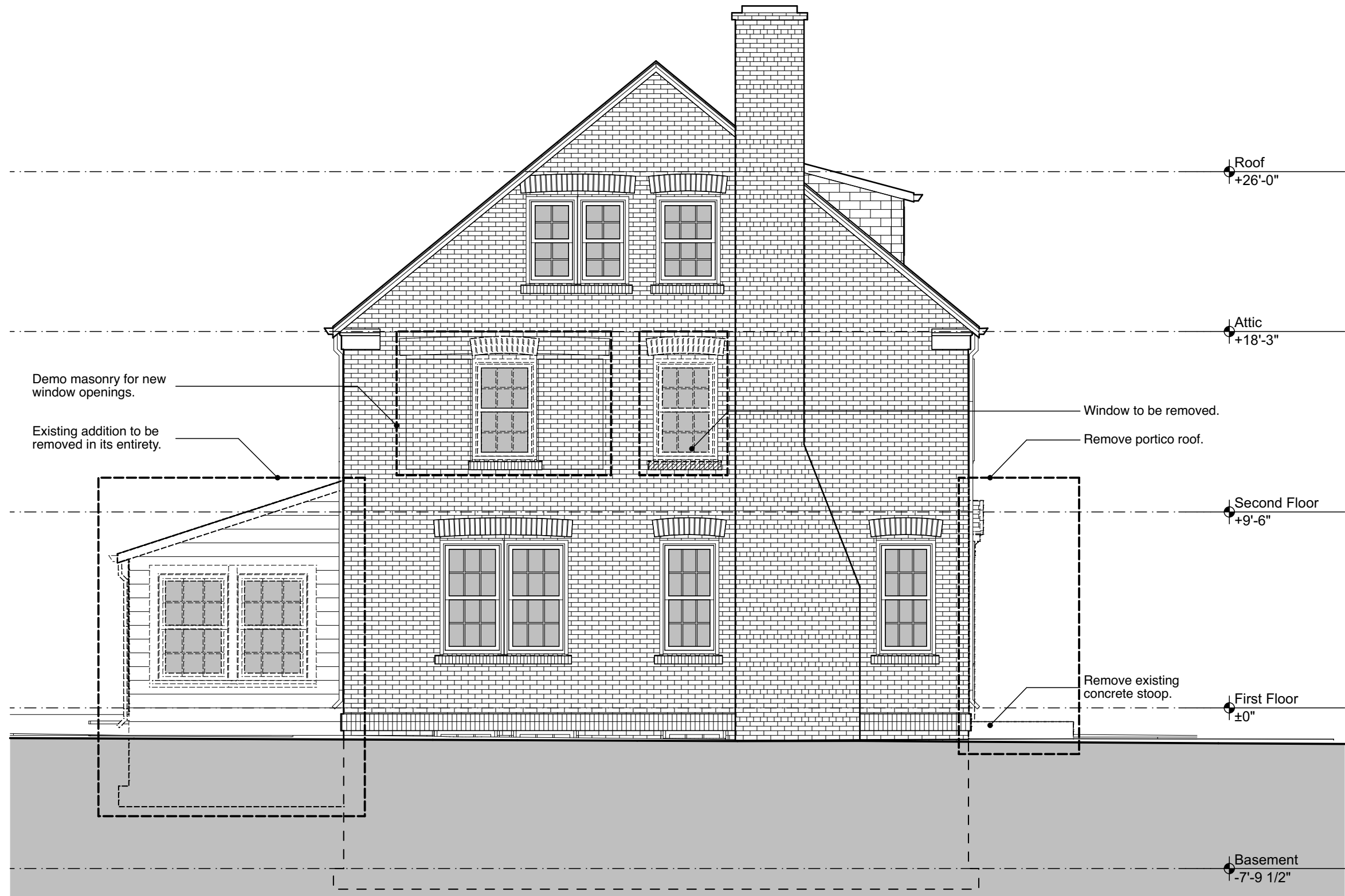
1 EAST (Side) Demolition Elevation SCALE: 3/16" = 1'-0"
