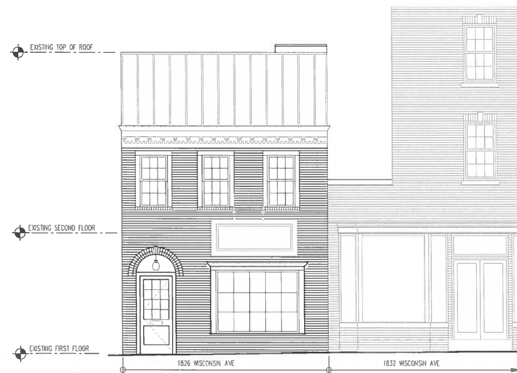
1 EXISTING FRONT ELEVATION 1/4"=1'-0"
