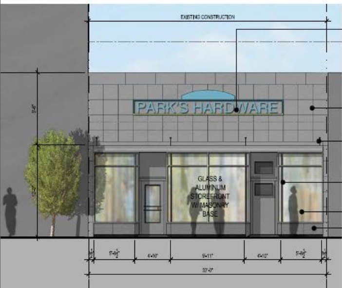
1 EXISTING RENDERED ELEVATION W/ AWNING REMOVED SCALE: 1/8" = 1'
