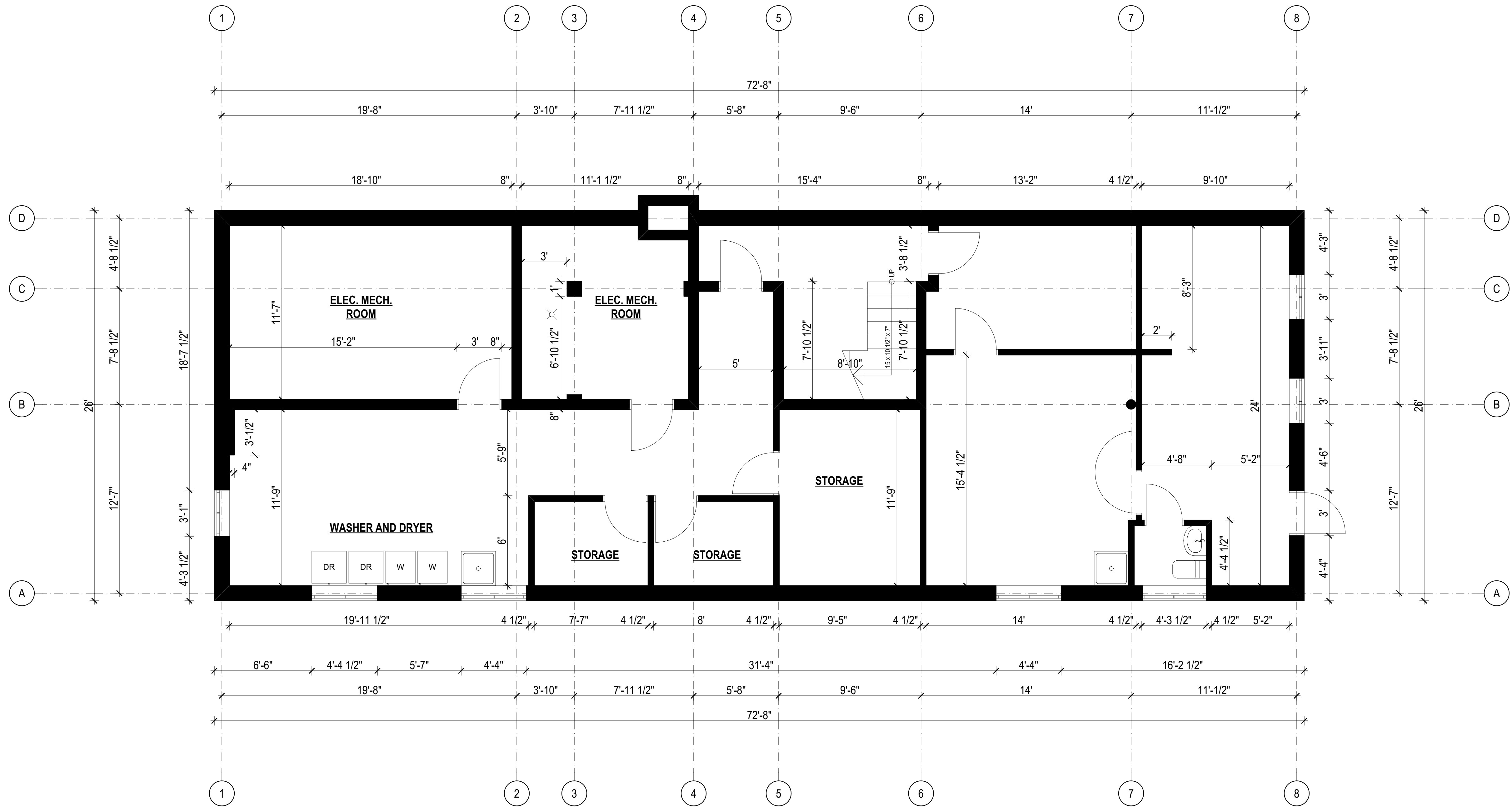
1 A-071 BASEMENT PLAN - EXISTING Scale: 1/4" = 1'-0"
