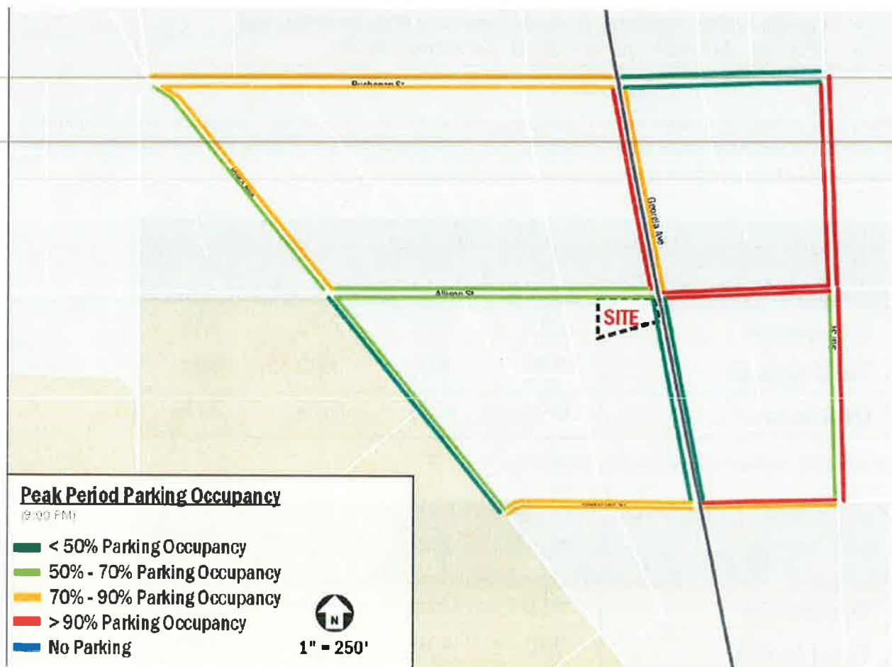
Figure 3: Peak Period Street Occupancy (Source: Gorove/ Slade)
